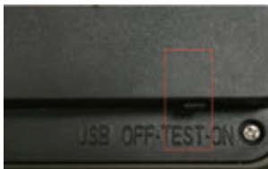
③ Switch to TEST
