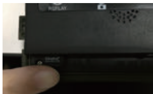
② Insert Micro SD card
