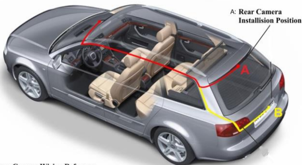
Rear Camera Wiring Reference (as shown above)
