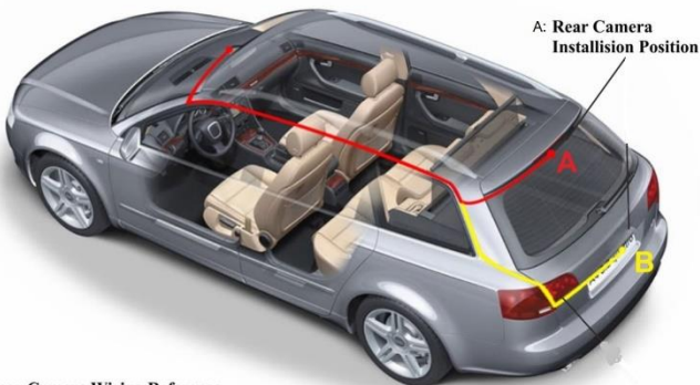
Rear Camera Wiring Reference (as shown above)
