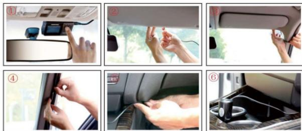
1. Choose the best installation position, stick pedestal bracket to window, fix it well, then we start wiring.
