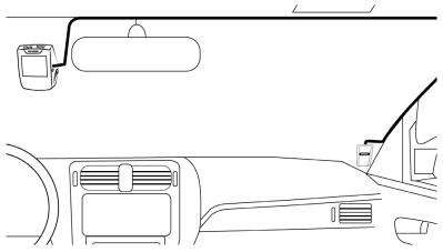
First, connect the GPS Logger to the port on the dash cam labeled "GPS".
