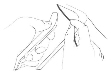
Once the GPS Logger is mounted, you can hide the connection to the dash cam by tucking the wire into the frame of your vehicle.
