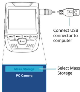
After the device powers up, press the OK Button to select Mass Storage. On the computer, navigate to device drive. The videos are stored at: \CARDVA MOVIE.
