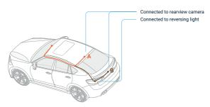
The rearview camera has two wire routing options as shown in the above figure. The first part of both options is characterized with concealing the wire routing against the edges of the door(s).
