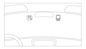
Once the dash cam is attached on the windshield with the included adhesive mount, place the motion sensor on the top of the windshield about a few inches away from the dash cam.
