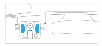
Finally, connect the power cable to the dash cam. Please DO NOT enable the parking monitor function in the settings of the dash cam. The motion sensing will automatically on once the vehicle is powered off.
