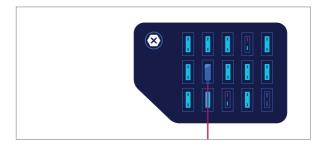
Find the switched fuse and connect the RED cable to it. This fuse has power only when the car is on.
