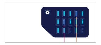
Find the hot fuse the connect the YELLOW cable to that. This fuse has power at all time.
