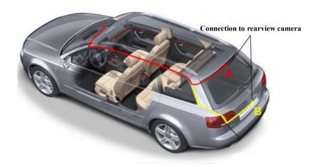
For the rearview camera, there are two wiring options as shown in the above figure. The first part of both options is characterized with concealed wire routing against the edges of the door(s).
