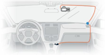
Plug Mini USB Connector to the Dashcam
