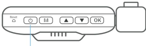
Press and hold the **Power** button to turn the device on manually
