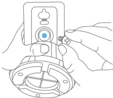
Step 2. Secure tightly with the stand screw
