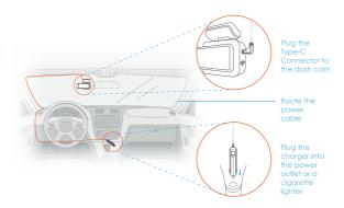
The camera will shut down after 3 seconds when it's disconnect from the power source and it should begin recording automatically the next time it is powered on.
