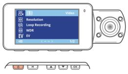
Press and hold the Power button to turn the device on manually
