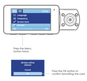
Use the **UP** and **DOWN** navigation buttons and go to the Format setting. Press the **OK** button to confirm the selection.
