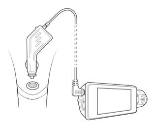
To format the memory card, make sure you have inserted your memory card, then turn on the device by connecting to a power source. Press **OK** to stop recording. Then press the **MENU** button twice to enter the System Setup Menu.
